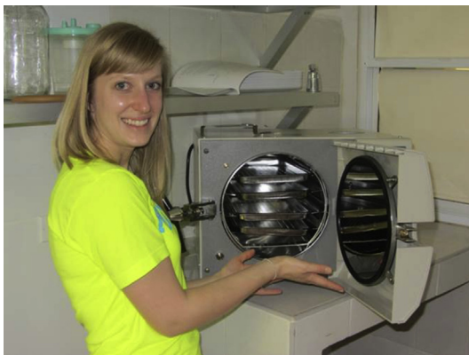
Fig. 18. One indispensable piece of equipment is the Automatic Autoclave Sterilizer purchased for your mission clinic in a size large enough to handle cranio-maxillofacial instrument sets and which can be set and operated by relatively inexperienced volunteer help so as to run constantly and assist in rapid instrument turnover, greatly enhancing the potential number of surgical cases handled each clinic. Care is to be given to use distilled water only and to review manufacturer's recommended usage with the team ahead of the busy operating day.
